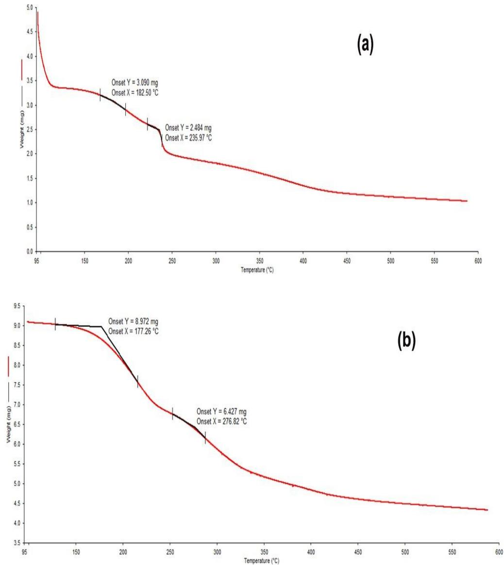
Figure 2. Degradation Time of the Biocomposite Films from kC (a) and kC/ZnONps (b) kC/ZnONps exhibited unique degradation time than the kC alone. Between 95-150 the biocomposite film from kC started to degrade rapidly and lost approximately 1.5mg of mass and continue as the temperature increases (a). The kC/ZnONps started to degrade at 150-200. This only implies that the incorporated ZnONps to the
