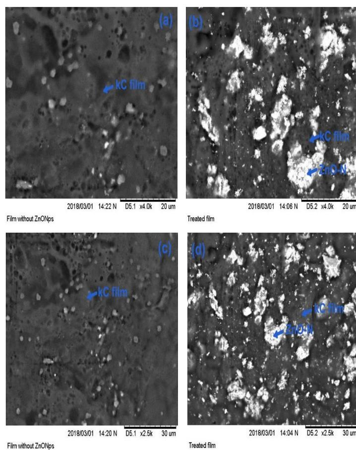
Figure 5. SEM Micrograph of the kC film without ZnONps (a) magnification =4,000, (c) magnification =2,500. The films with ZnONps (b) magnification = 4,000, and (d) Magnification = 2,500
