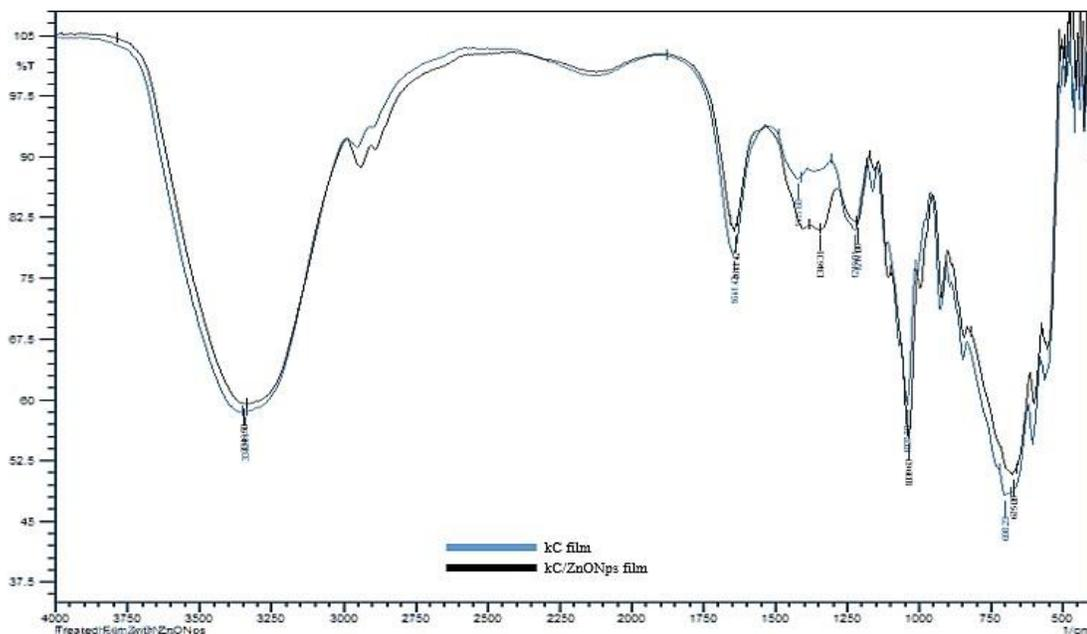
The structural formation analysis produced by FTIR showed that there were no changes on the peaks of the films. The functional group alcohol (-OH) was present in both film samples. The functional group present in both films are the same but as we can observe, there is a sequence between the peaks observed. This may explain the structural composition of the film, biocomposite films with metal oxide have parallel peaks to kC alone. It was postulated that the ZnONps will only coat the kC
